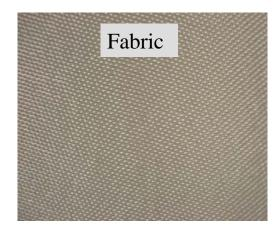
Fig. 1 S2-glass fiber, 8HS woven fabric single side coated with an aluminum alloy at a deposition of 0.37 g/ in<sup>2</sup>.
