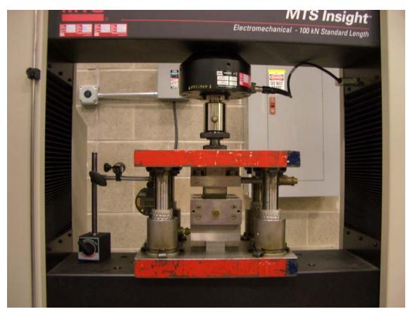
Fig. 2 Compaction test fixture.
